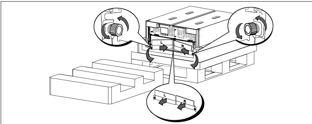
**7** Ensure all battery connectors are disconnected.
