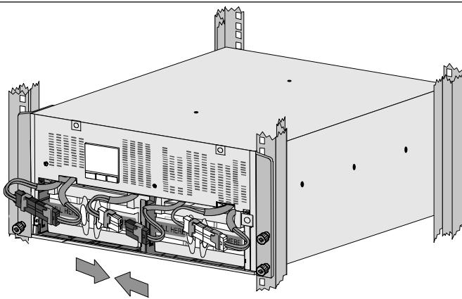
**10** Connect the internal battery connectors:
