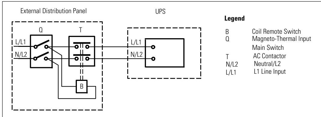
The following table lists backfeed protection devices (AC contactors) that can be used as an external isolating device for backfeed protection. Only use AC contactors listed in the table.
