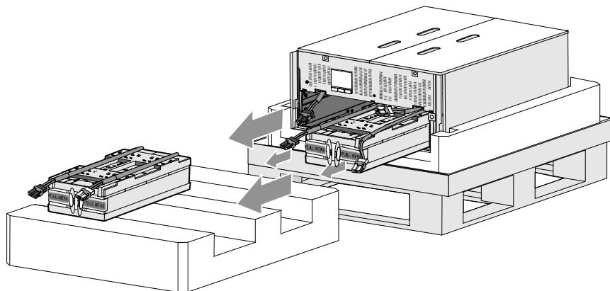
**!** **CAUTION:** The cabinet is heavy (46 kg/101 lb) with the batteries removed. Lifting the cabinet from the shipping carton requires a minimum of two people.
