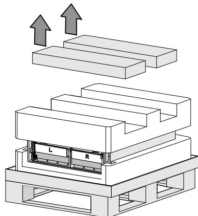
**5** Remove the top Styrofoam section and set it on a flat, stable surface nearby.
